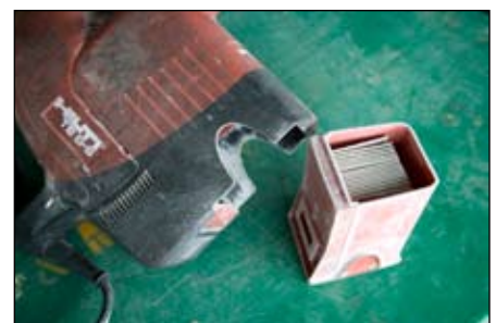
Drill with dust removal system
